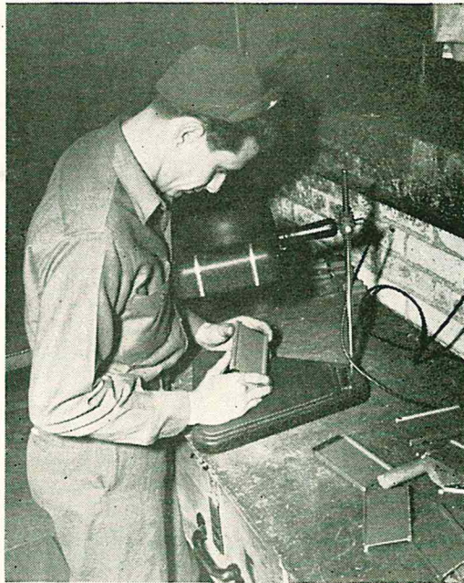
ED COLEMAN uses a magnifying glass to inspect Wheelabrator blade castings for blow holes, and other imperfections. He inspects all rough castings produced in our foundry. Such careful attention to accuracy is required by modern, precision machinery.
