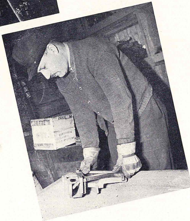
L. E. CRAMER uses a gauge to inspect rough link castings. If this gauge does not slip easily around the part, the casting is rejected. He inspects all rough castings produced outside our plant.
