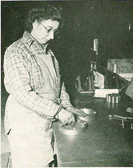
SOPHIE BURKHART inspects spacer rings. On this one part she checks the inside taper, the length and width of the ring, and the holes, to be sure they are properly spaced. She, as the other inspectors, reads drawings to learn the proper dimensions of the parts.
