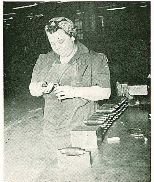
CLARA HEINTZ uses a micrometer to check Wheelabrator wheel spacers. The gauge in the foreground checks the body and ends of the spacer. The women inspect the small, light weight parts, while the men work on the heavy pieces.
