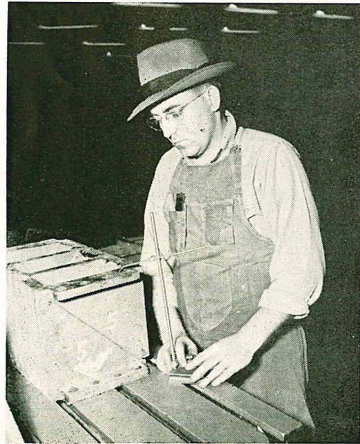
DICK ATKISON, gang leader, checks the height of this Rod Machine casting die, with the aid of a surface gauge. To help in the accurate inspection of material, this department has a large number of gauges and instruments.
